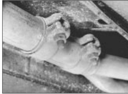
19.2 Check exhaust system connections for leaks and security
