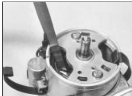
16.10a Checking contact breaker points gap
