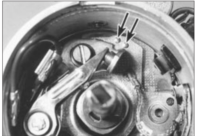
16.10c Two pips and notch (arrowed) for inserting screwdriver when adjusting contact breaker points gap
