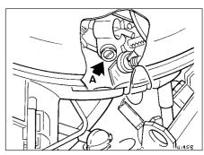
15.37b Idle speed adjusting screw (A) from July 1985
