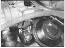
16.10 Fast idle speed adjustment screw (2)
