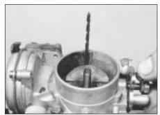
15.3a Checking choke valve gap with twist drill
