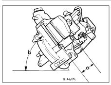
15.36 Float level checking diagram  $a = 28 \pm 1.0 \text{ mm}$   $b = 45^{\circ}$  angle
