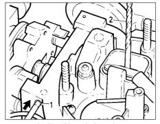
16.2b Checking choke valve gap
