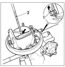
15.53 Checking choke valve gap (wide open kick)
