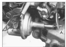
17.39b Fast idle adjustment screw (A)
