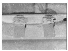
7.9 Fuel tank retaining strap-to-floor bolts
