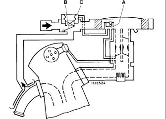
4.2 Air cleaner load and temperature control diagram – 1.05 and 1.3 litre
