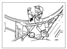
15.22 Idle speed adjustment screw location
