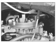
3.3a Disconnecting temperature sensor hose . . .
