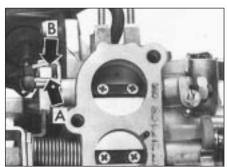
17.15 Lock lever clearance with throttle valves closed
