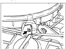
15.26 Mixture (CO content) adjustment screw location
