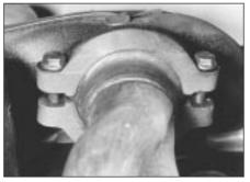
19.10 Exhaust downpipe-to-manifold flange connection - 1.3 litre
