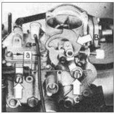
12.9 Choke cable adjustment setting – 1.05 litre
