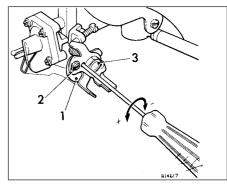
15.57 Accelerator pump adjustment
