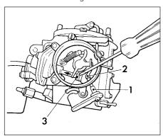
15.40 Choke valve gap adjustment
