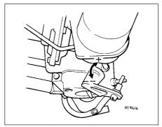
15.54 Adjusting choke valve gap (wide open kick)
