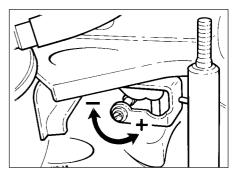
15.6 Accelerator pump adjuster screw
