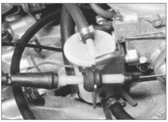
10.4 Release cable grommet from support bracket
