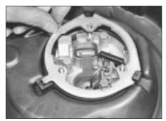
3.2 Removing air cleaner body retaining ring - 1.3 litre
