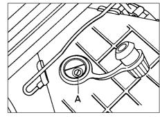
17.34b Mixture (CO) adjustment screw (A)
