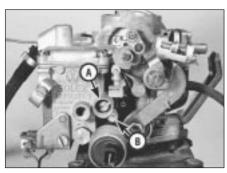
15.10 Idle speed (A) and mixture (B) adjusting screw locations
