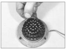
18.3c Removing sealing ring from heater element
