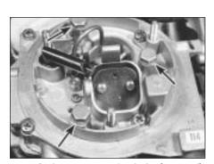
13.8 Carburettor securing bolts (arrowed)Pierburg/Solex 2E3
