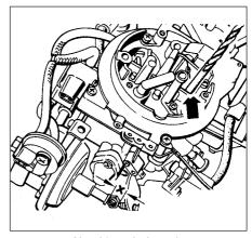
17.5 Checking choke valve gap
