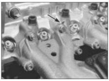
19.6 Inlet manifold-to-cylinder head securing nuts and bolts
