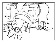
15.32 Accelerator pump adjustment
