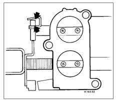
16.7b Locking lever clearance with throttle valves closed
