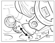
16.3 Accelerator pump adjustment
