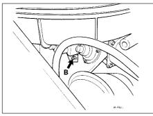
15.37c Mixture (CO content) adjusting screw (B)
