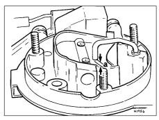
15.20 Enrichment tube adjustment  $a = 1.0 \pm 0.3 \text{ mm}$
